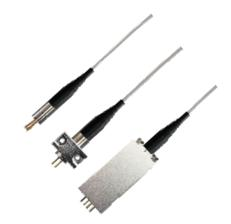
The FPLD series fiber-coupled laser diodes are designed with a GaAs quantum well structure. These diodes feature a built-in photodiode for precise monitoring and feedback control of the laser's output power. Housed in standard TO packages, these diodes are pigtailed to a 1-meter long single-mode fiber terminated with an FC/APC connector. Each unit undergoes rigorous testing prior to shipment to ensure reliability.
